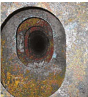
Pre-treatment with FLUID FILM Liquid A with 25 µm (wff.)
